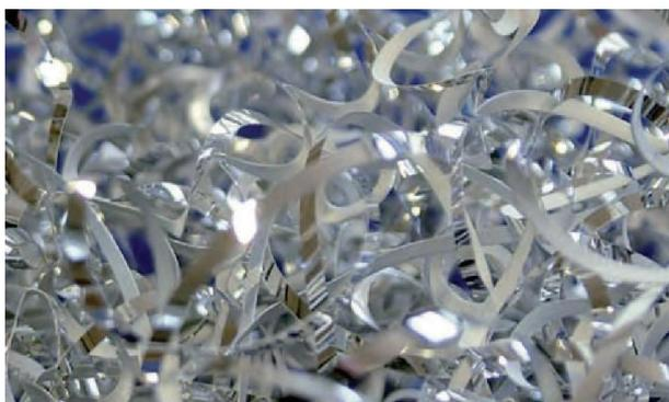
Without 3D-chip breaker: Flow chips
