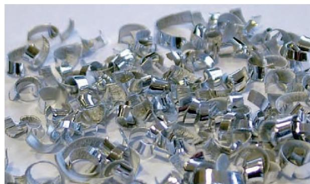
With 3D-chip breaker: Breakage chips
